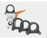
The Offset Link is compatible with all HYTORC The Offset Link provides an interchangeable Hydraulic, Pneumatic and Electric Torque tools. The Offset Link comes in two basic drive types compatible with either 3/4" and 1" square drives. The torque multiplication factor for each cartridge is clearly marked; simply multiply the factor by the desired torque and set the torque on the tool for accurate and repeatable bolting operations.
