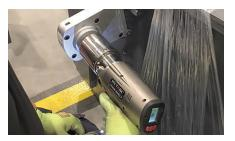
cartridge system that allows the user to easily change out cartridges in the field to accommodate a range of hex sizes. The Offset Link is compatible with the HYTORC Washer which eliminates bending and side load while increasing the safety and speed of all bolting operations.
