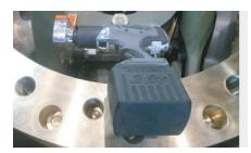
The Offset Link provides a convenient low-profile extension that allows squaredrive tools to reach bolts that are otherwise difficult to access because of obstructions. The links essentially allow the square drive tool to function as a low-clearance tool thereby eliminating the need for additional tooling. This bolting configuration is ideal for tightening fasteners with protruding bolts.
