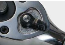
The Ratchet Reversing Lever quickly and conveniently changes the ratcheting direction. The lever has three positions: Clockwise, Counter-Clockwise, and Locked.
